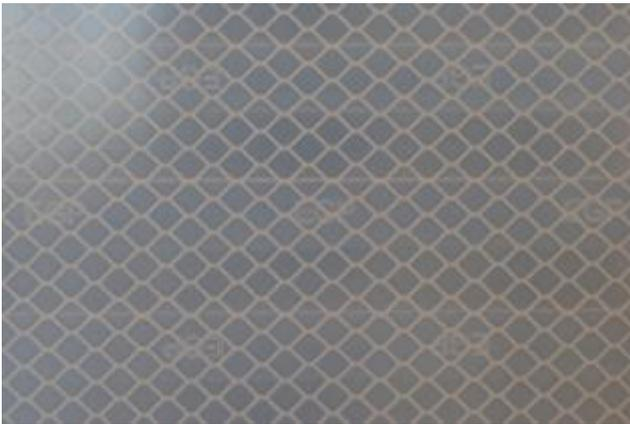
The Engineer Grade Prismatic sheeting is differentiated from other prismatic or encapsulated lens sheeting by the distinctive surface pattern and the visible integral 'EGP' marking.
